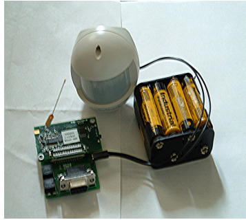
Figure 7: PIR sensor interfaced with mote
