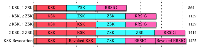
Figure 3: DNSKEY response sizes during the rollover.
