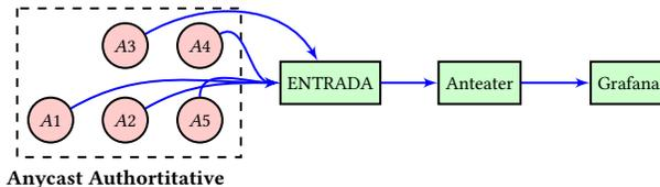
Figure 1: DNS TCP Latency Monitoring Architecture
