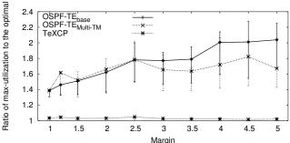
Figure 5: When traffic deviates from TM by a margin, TeXCP stays within a few percent of the optimal max-utilization; OSPF-TE  $_{Base}$  and OSPF-TE  $_{Multi-TM}$  lead to much larger max-utilization.
