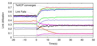
Figure 10: Changes in link utilization during TeXCP convergence for a representative sample of links in the Sprint topology. Both the maximum utilization in the network and the individual link utilization converge smoothly without oscillations.
