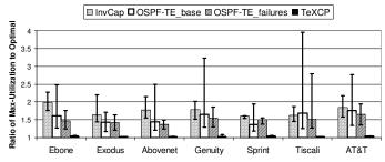
Figure 6: Under failures, TeXCP's max-utilization is within a few percent of the optimal; InvCap, OSPF-TE $_{Base}$ , and OSPF-TE $_{Failures}$  become highly suboptimal. Figure shows the 90th percentile (thick) and maximums (thin) taken over multiple TMs.
