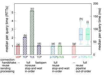
Fig. 6: Per-query response times for 140 repeated queries with different protocols, measured in RTTs (left axis) and ms (right). (Medians; boxes add quartiles.)
