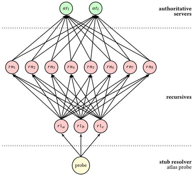
**Figure 17: probe 284777 on dataset i. all  $r1$ 's are connected to all  $rn$ 's, which are connected to all  $at$ 's.**
