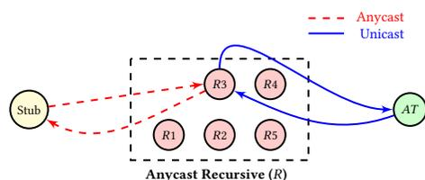
Figure 2: Stub resolver and Anycast Recursive
