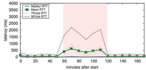
(b) Experiment F: 75% packet loss (1800 s TTL)
