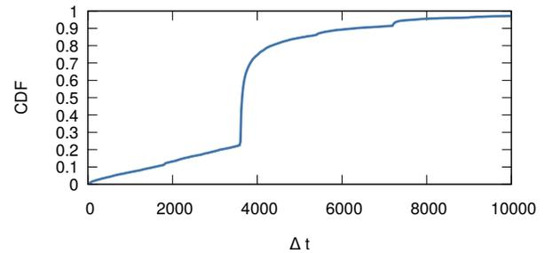
**Figure 4: ECDF of the median  $\Delta t$  for recursives with at least 5 queries to ns1-ns5.dns.nl (TTL of 3600 s.)**
