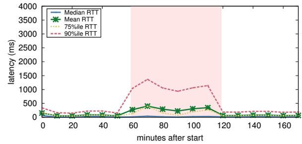
(a) Experiment E: 50% packet loss (1800 s TTL)
