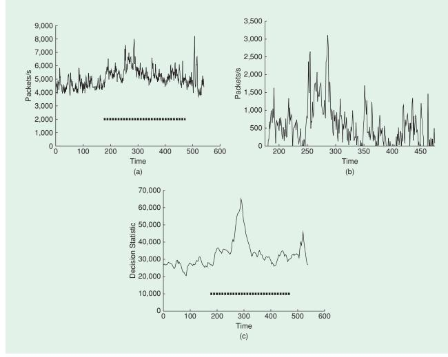
[FIG1] A low-volume attack of 670 packets per second is detected using change-point detection on the spectral content of the aggregate network traffic. (a) Aggregate network traffic in packets per second. Attack duration indicated by the line. (b) Attack traffic in packets per second. (c) Attack is detected using nonparametric detection techniques. Attack duration indicated by the line.
