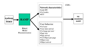
Figure 1: Data flow of RAMP
