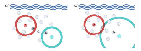
Figure 3. Illustration of space-time volume (adapted from ([23], fig. 1)): long acoustic latencies mean that packets from A and E are successfully received at B and D in part (a), even though they are sent concurrently, while in part (b), packets collide at B even though they are sent at different times. (a) Same transmission time, no collision; (b) different transmission time but collision at B. (Online version in colour.)
