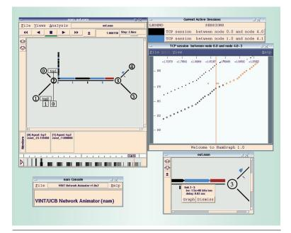
Figure 2. A typical nam session. The top-left window shows a packet animation for a network, with monitors and statistics running across the bottom. The top-right window shows TCP flows in the trace. The center-right window shows a time-sequence plot of a specific TCP flow. The bottom-right window shows a zoomed view of the packet animation and a pop-up query concerning link 2-3. The bottom-left window is the console for nam-wide operations.
