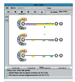
Figure 3. Using packet animation in nam. Here nam is comparing three different TCP protocols with the same workload. The different numbers of packets in flight and the packet loss in the top variant represent variations in the three protocols.
