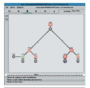
Figure 5. Visualization of applications with nam. The shapes represent node types—the hexagons are the client and server and the circles are caches. The node color shows the cache status; rings around nodes show algorithm status.
