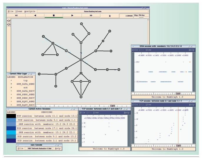
Figure 6. Nam provides time-event graphs, which aid specific investigations. The bottom center and bottom right windows show TCP time-sequence number graphs. The top right window shows a plot of SRM events against time.
