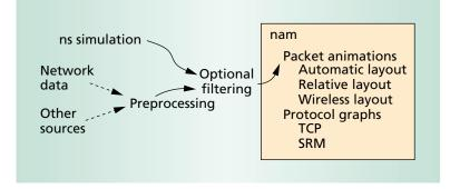
Figure 1. Data flows into nam from network data or other sources after preprocessing into the nam trace format. Optional filtering adds information to a nam trace, possibly highlighting specific flows or generating additional statistics.
